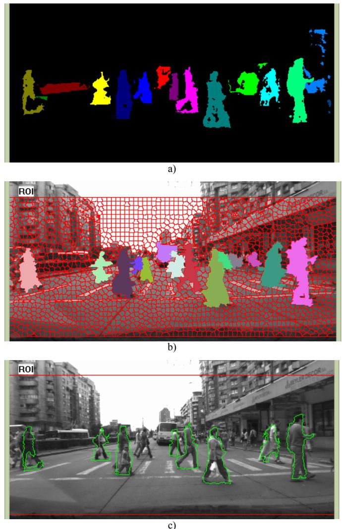
Figure 8. Pedestrian hypotheses shapes: a) 3D points grouping (random color for each hypothesis); b) segmentation based on stereo and superpixels; c) contours based on the 3D points groups
