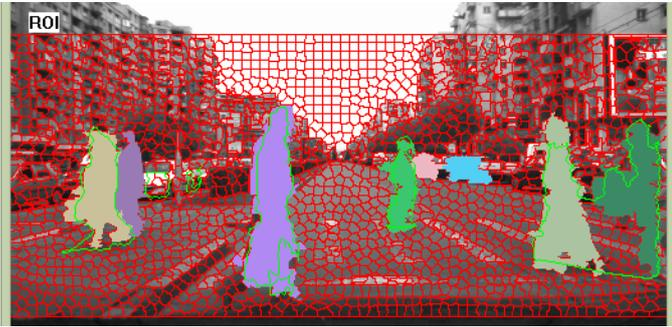
Figure 4. Superimposing the extracted contour (with green color) based on the 3D points over the superpixels regions of pedestrian hypotheses
