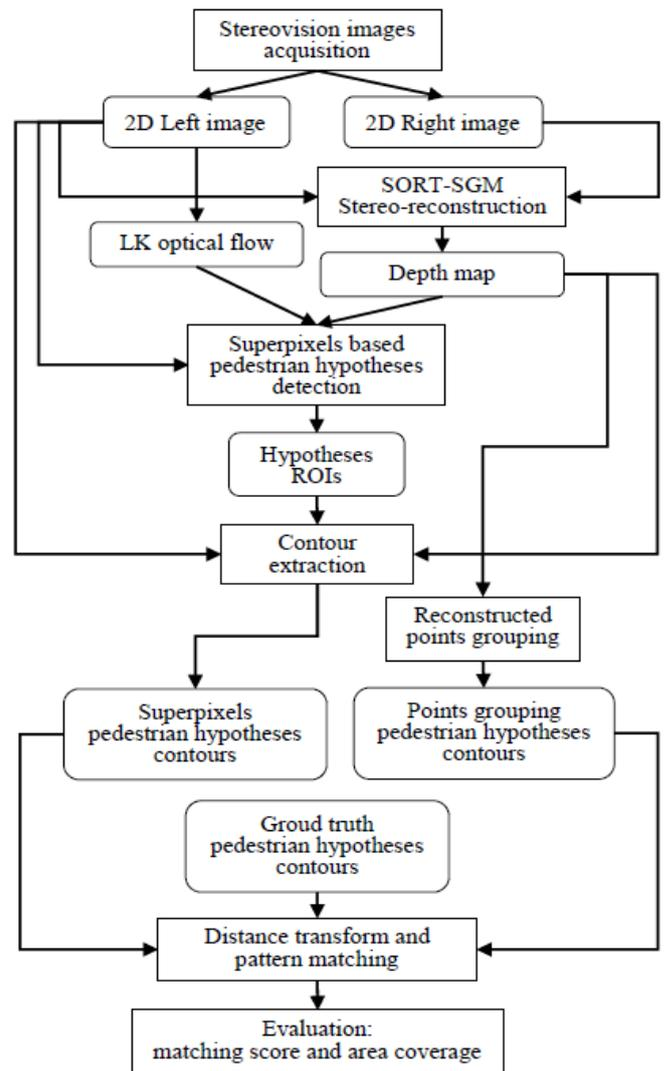
Figure 1. Superpixels and stereo based pedestrian hypotheses contour extraction and validation system architecture
